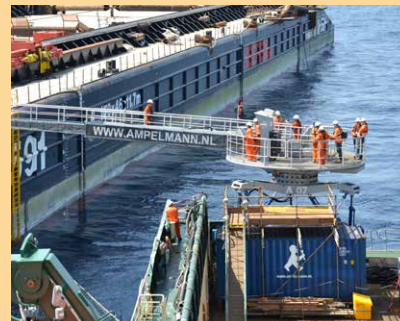
An Ampelmann dynamically stabilized gangway in use
